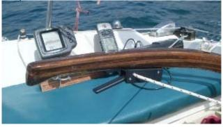
I found I could lock the tiller for a few seconds while trimming without a serious course change. This gave me a way to let go, just for a couple of seconds, and attend to a task like trimming the guy. I definitely liked having the device hooked up when short handed in the cockpit.
