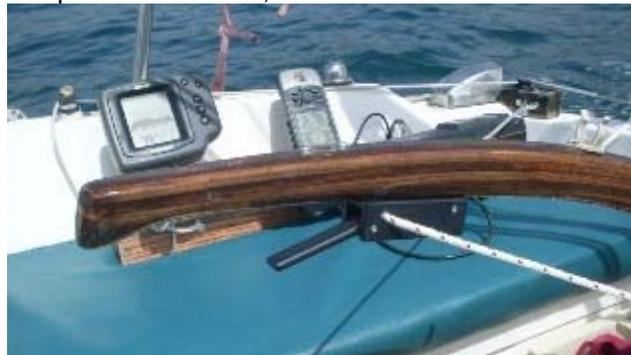
I found I could lock the tiller for a few seconds while trimming without a serious course change. This gave me a way to let go, just for a couple of seconds, and attend to a task like trimming the guy. I definitely liked having the device hooked up when short handed in the cockpit.
